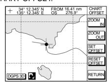
Figure 10-2 Plotter display, chart offset selected
